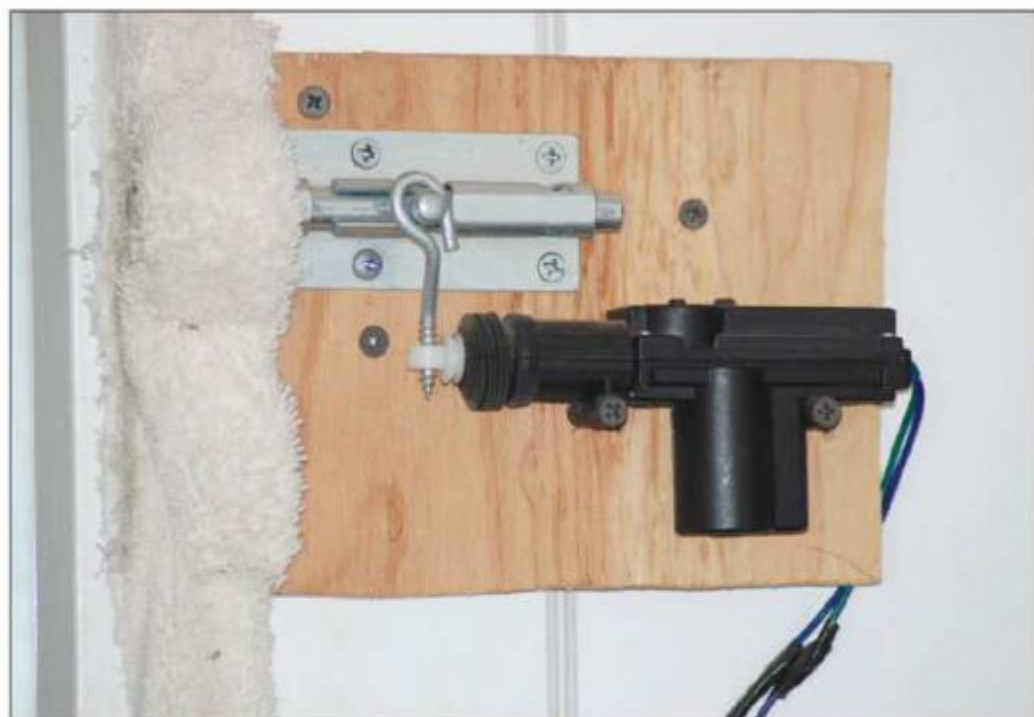
Left: A remote-activated double-deadbolt door-locking system. Above: A close-up of the actuator and deadbolt mechanism.
